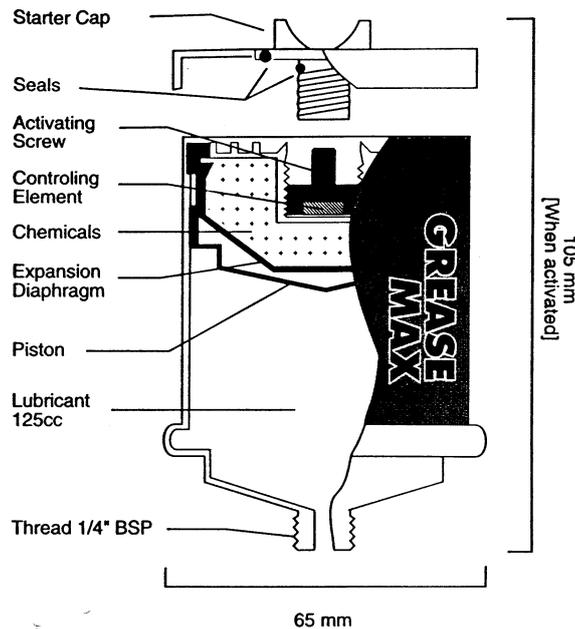
**GreaseMax** requires a minimum of approximately 8 hours for a type 1 unit to approximately 40 hours for a type 12 unit to develop sufficient internal pressure to commence discharging lubricant. This period is normally not a problem for well maintained bearings however if lubrication is required in less than the start up period then activate **GreaseMax** in advance.
